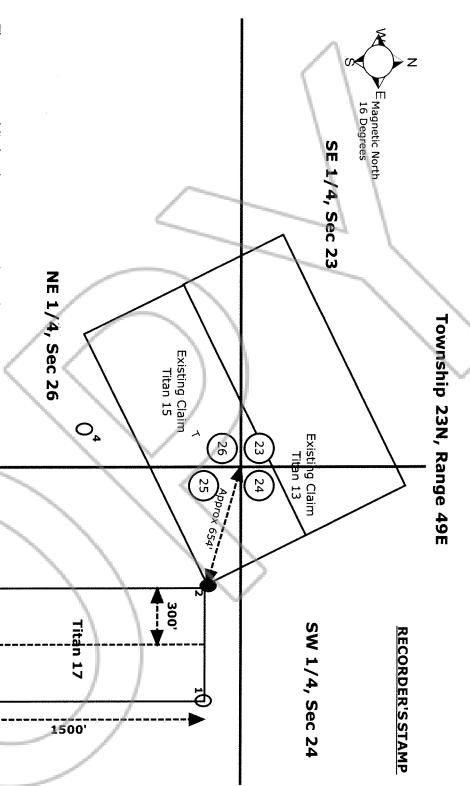
The nearest public land survey point lies whereas, the corner #2 of Titan #17 is approximately 654' from the common corner of sections 23, 24, 25 and 26. The common border of 24 and 25 is approx. 195' North of the claim and the common border of 23 and 26 is approx. 648' West of the claim.
