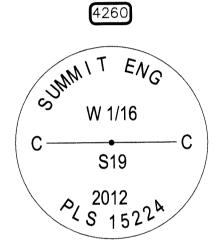
CENTER WEST SIXTEENTH CORNER OF SECTION 19, T22N, R51E, MDM. NOTHING FOUND. ESTABLISHED BY SINGLE PROPORTIONATE MEASUREMENT COMPUTATION. SET 5/8" REBAR WITH 2" DIAMETER ALUMINUM CAP WITH MARKINGS AS SHOWN TO THE LEFT. TOP OF CAP IS FLUSH WITH THE GROUND IN AREA OF LOW BRUSH, JUNIPERS, & PINIONS. SET T-POST 1' NORTH OF CORNER.
