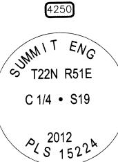
CENTER QUARTER OF SECTION 19, T22N, R51E, MDM. NOTHING FOUND. ESTABLISHED BY EXTENDING THE BEARING OF THE EAST LINE OF THE SOUTHEAST QUARTER (#4110 TO #4040) FROM THE SOUTH QUARTER CORNER (#4100) TO INTERSECT THE EAST/WEST CENTERLINE OF THE SECTION (#4040 TO #4050). SET 5/8" REBAR WITH 2" DIAMETER ALUMINUM CAP WITH MARKINGS AS SHOWN TO THE LEFT. TOP OF CAP IS 1" ABOVE THE GROUND IN AREA OF LOW BRUSH, JUNIPERS, & PINIONS. SET T-POST 1' NORTH OF
