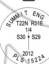
QUARTER CORNER COMMON TO SECTION 29 AND SECTION 30, T22N, R51E, MDM. FOUND 4"X4"X3.25' WEATHERED WOOD POST LAYING ON THE GROUND IN A NE/SW DIRECTION. NO SUBSURFACE EVIDENCE OF WOOD POST WAS FOUND. ACCEPTED AS THE ORIGINAL MONUMENT HOLDING THE NORTHEAST END OF THE WOOD POST. SET 5/8" REBAR WITH 2" DIAMETER ALUMINUM CAP WITH MARKINGS AS SHOWN TO THE LEFT. TOP OF CAP IS 1" BELOW THE GROUND IN AN AREA OF LOW BRUSH. SET T-POST 1' NORTH OF CORNER.
