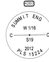
CENTER WEST SIXTEENTH CORNER OF SECTION 19, T22N, R51E, MDM. NOTHING FOUND. ESTABLISHED BY SINGLE PROPORTIONATE MEASUREMENT COMPUTATION. SET 5/8" REBAR WITH 2" DIAMETER ALUMINUM CAP WITH MARKINGS AS SHOWN TO THE LEFT. TOP OF CAP IS FLUSH WITH THE GROUND IN AREA OF LOW BRUSH, JUNIPERS, & PINIONS. SET T-POST 1' NORTH OF CORNER.
