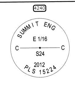
CENTER EAST SIXTEENTH CORNER OF SECTION 24, T22N, R50E, MDM. NOTHING FOUND. ESTABLISHED BY BREAKDOWN OF THE SECTION. SET 5/8" REBAR WITH 2" DIAMETER ALUMINUM CAP WITH MARKINGS AS SHOWN TO THE LEFT. TOP OF CAP IS FLUSH WITH GROUND IN AREA OF LOW SAGE. SET T-POST 1' NORTH OF CORNER.
