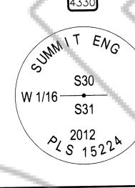
WEST SIXTEENTH CORNER COMMON TO SECTION 30 AND SECTION 31, T22N, R51E, MDM. NOTHING FOUND. ESTABLISHED BY SINGLE PROPORTIONATE MEASUREMENT COMPUTATION. SET 5/8" REBAR WITH 2" DIAMETER ALUMINUM CAP WITH MARKINGS AS SHOWN TO THE LEFT. TOP OF CAP IS FLUSH WITH GROUND IN AREA OF LOW SAGE. SET T-POST 1' NORTH OF CORNER.
