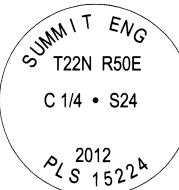
CENTER QUARTER OF SECTION 24, T22N, R50E, MDM. NOTHING FOUND. ESTABLISHED BY BREAKDOWN OF THE SECTION. SET 5/8" REBAR WITH 2" DIAMETER ALUMINUM CAP WITH MARKINGS AS SHOWN TO THE LEFT. TOP OF CAP IS FLUSH WITH GROUND IN AREA OF LOW SAGE. SET T-POST 1' NORTH OF CORNER.
