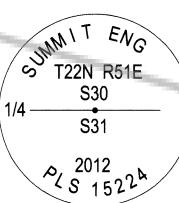
QUARTER CORNER COMMON TO SECTION 30 AND SECTION 31, T22N, R51E, MDM. FOUND FIVE 5" LONG DETERIORATED WOOD POST REMNANTS LAYING IN A 6' DIAMETER AREA. NO SUBSURFACE EVIDENCE OF WOOD POST WAS FOUND. ACCEPTED AS THE ORIGINAL MONUMENT HOLDING THE LARGEST OF THE WOOD REMNANTS (MOST NORTHERLY). SET 5/8" REBAR WITH 2" DIAMETER ALUMINUM CAP WITH MARKINGS AS SHOWN TO THE LEFT. TOP OF CAP IS 1" ABOVE THE GROUND IN AN AREA OF LOW SAGE. SET T-POST 1' NORTH OF CORNER.
