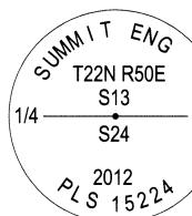
QUARTER CORNER COMMON TO SECTION 13 AND SECTION 24, T22N, R50E, MDM. NO ORIGINAL EVIDENCE FOUND. ESTABLISHED BY SINGLE PROPORTIONATE MEASUREMENT COMPUTATION. SET 5/8" REBAR WITH 2" DIAMETER ALUMINUM CAP WITH MARKINGS AS SHOWN TO THE LEFT. TOP OF CAP IS 1" ABOVE THE GROUND IN AN AREA OF LOW SAGE. SET T-POST 1' NORTH OF CORNER.
