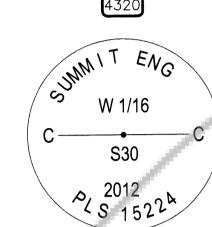
CENTER WEST SIXTEENTH CORNER OF SECTION 30, T22N, R51E, MDM. NOTHING FOUND. ESTABLISHED BY SINGLE PROPORTIONATE MEASUREMENT COMPUTATION. SET 5/8" REBAR WITH 2" DIAMETER ALUMINUM CAP WITH MARKINGS AS SHOWN TO THE LEFT. TOP OF CAP IS FLUSH WITH GROUND IN PREVIOUSLY CULTIVATED AREA. SET T-POST 1' NORTH OF CORNER.
