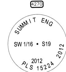
SOUTHWEST SIXTEENTH CORNER OF SECTION 19, T22N, R51E, MDM. NOTHING FOUND. ESTABLISHED BY BREAKDOWN OF THE SECTION. SET 5/8" REBAR WITH 2" DIAMETER ALUMINUM CAP WITH MARKINGS AS SHOWN TO THE LEFT. TOP OF CAP IS FLUSH WITH GROUND IN PREVIOUSLY CULTIVATED AREA. SET T-POST 1' NORTH OF CORNER.
