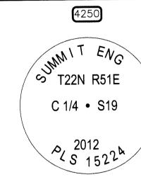
CENTER QUARTER OF SECTION 19, T22N, R51E, MDM. NOTHING FOUND. ESTABLISHED BY EXTENDING THE BEARING OF THE EAST LINE OF THE SOUTHEAST QUARTER (#4110 TO #4040) FROM THE SOUTH QUARTER CORNER (#4100) TO INTERSECT THE EAST/WEST CENTERLINE OF THE SECTION (#4040 TO #4050). SET 5/8" REBAR WITH 2" DIAMETER ALUMINUM CAP WITH MARKINGS AS SHOWN TO THE LEFT. TOP OF CAP IS 1" ABOVE THE GROUND IN AREA OF LOW BRUSH, JUNIPERS, & PINIONS. SET T-POST 1' NORTH OF CORNER.
