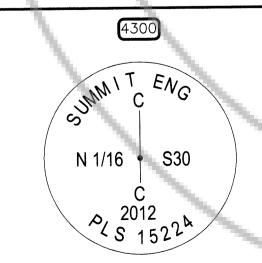
CENTER NORTH SIXTEENTH CORNER OF SECTION 30, T22N, R51E, MDM. NOTHING FOUND. ESTABLISHED BY BREAKDOWN OF THE SECTION. SET 5/8" REBAR WITH 2" DIAMETER ALUMINUM CAP WITH MARKINGS AS SHOWN TO THE LEFT. TOP OF CAP IS FLUSH WITH GROUND IN PREVIOUSLY CULTIVATED AREA. SET T-POST 1' NORTH OF CORNER.
