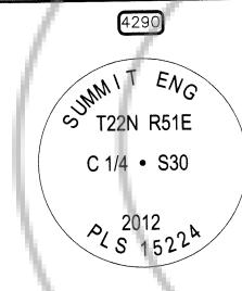
CENTER QUARTER OF SECTION 30, T22N, R51E, MDM. NOTHING FOUND. ESTABLISHED BY BREAKDOWN OF THE SECTION. SET 5/8" REBAR WITH 2" DIAMETER ALUMINUM CAP WITH MARKINGS AS SHOWN TO THE LEFT. TOP OF CAP IS FLUSH WITH GROUND IN AREA OF LOW SAGE. SET T-POST 1' NORTH OF CORNER.
