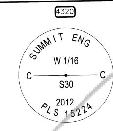
CENTER WEST SIXTEENTH CORNER OF SECTION 30, T22N, R51E, MDM. NOTHING FOUND. ESTABLISHED BY SINGLE PROPORTIONATE MEASUREMENT COMPUTATION. SET 5/8" REBAR WITH 2" DIAMETER ALUMINUM CAP WITH MARKINGS AS SHOWN TO THE LEFT. TOP OF CAP IS FLUSH WITH GROUND IN PREVIOUSLY CULTIVATED AREA. SET T-POST 1' NORTH OF CORNER.
