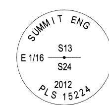
EAST SIXTEENTH CORNER COMMON TO SECTION 13 AND SECTION 24, T22N, R50E, MDM. NOTHING FOUND. ESTABLISHED BY BREAKDOWN OF THE SECTION. SET 5/8" REBAR WITH 2" DIAMETER ALUMINUM CAP WITH MARKINGS AS SHOWN TO THE LEFT. TOP OF CAP IS FLUSH WITH GROUND IN AREA OF A DRY POND. SET T-POST 1' NORTH OF CORNER.
