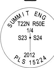
QUARTER CORNER COMMON TO SECTION 23 AND SECTION 24, T22N, R50E, MDM. NOTHING FOUND. ESTABLISHED BY SINGLE PROPORTIONATE MEASUREMENT COMPUTATION. SET 5/8" REBAR WITH 2" DIAMETER ALUMINUM CAP WITH MARKINGS AS SHOWN TO THE LEFT. TOP OF CAP IS FLUSH WITH THE GROUND IN AN AREA OF SAGE AND JUNIPERS. CORNER IS LOCATED APPROXIMATELY 2' EAST OF A SMALL DRAINAGE. SET T-POST 1 NORTH OF CORNER.
