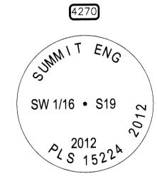
SOUTHWEST SIXTEENTH CORNER OF SECTION 19, T22N, R51E, MDM. NOTHING FOUND. ESTABLISHED BY BREAKDOWN OF THE SECTION. SET 5/8" REBAR WITH 2" DIAMETER ALUMINUM CAP WITH MARKINGS AS SHOWN TO THE LEFT. TOP OF CAP IS FLUSH WITH GROUND IN PREVIOUSLY CULTIVATED AREA. SET T-POST 1' NORTH OF CORNER.
