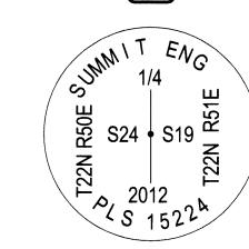
QUARTER CORNER BETWEEN SECTION 24, T22N, R50E, MDM., AND SECTION 19, T22N, R51E, MDM. NO ORIGINAL EVIDENCE FOUND. ESTABLISHED BY SINGLE PROPORTIONATE MEASUREMENT COMPUTATION ALONG THE RANGE LINE (FROM #4020 TO #4170). SET 5/8" REBAR WITH 2" DIAMETER ALUMINUM CAP WITH MARKINGS AS SHOWN TO THE LEFT. TOP OF CAP IS FLUSH WITH GROUND IN PREVIOUSLY CULTIVATED AREA. SET T-POST 1' NORTH OF CORNER.
