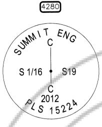
CENTER SOUTH SIXTEENTH CORNER OF SECTION 19, T22N, R51E, MDM. NOTHING FOUND. ESTABLISHED BY BREAKDOWN OF THE SECTION. SET 5/8" REBAR WITH 2" DIAMETER ALUMINUM CAP WITH MARKINGS AS SHOWN TO THE LEFT. TOP OF CAP IS 1" ABOVE GROUND IN AREA OF LOW BRUSH, JUNIPERS, & PINIONS. SET T-POST 1' NORTH OF CORNER.
