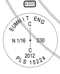
CENTER NORTH SIXTEENTH CORNER OF SECTION 30, T22N, R51E, MDM. NOTHING FOUND. ESTABLISHED BY BREAKDOWN OF THE SECTION. SET 5/8" REBAR WITH 2" DIAMETER ALUMINUM CAP WITH MARKINGS AS SHOWN TO THE LEFT. TOP OF CAP IS FLUSH WITH GROUND IN PREVIOUSLY CULTIVATED AREA. SET T-POST 1' NORTH OF CORNER.
