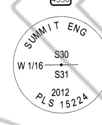
WEST SIXTEENTH CORNER COMMON TO SECTION 30 AND SECTION 31, T22N, R51E, MDM. NOTHING FOUND. ESTABLISHED BY SINGLE PROPORTIONATE MEASUREMENT COMPUTATION. SET 5/8" REBAR WITH 2" DIAMETER ALUMINUM CAP WITH MARKINGS AS SHOWN TO THE LEFT. TOP OF CAP IS FLUSH WITH GROUND IN AREA OF LOW SAGE. SET T-POST 1' NORTH OF CORNER.
