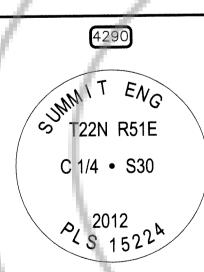
CENTER QUARTER OF SECTION 30, T22N, R51E, MDM. NOTHING FOUND. ESTABLISHED BY BREAKDOWN OF THE SECTION. SET 5/8" REBAR WITH 2" DIAMETER ALUMINUM CAP WITH MARKINGS AS SHOWN TO THE LEFT. TOP OF CAP IS FLUSH WITH GROUND IN AREA OF LOW SAGE. SET T-POST 1' NORTH OF CORNER.
